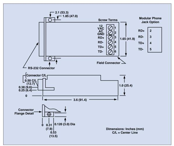
communicate at data rates up to 57,600 baud. A self-powered model and a host-powered model are available. The self-powered unit uses 12 Vac from a wall-mounted transformer while the host-powered unit takes ±DC power from pins 9 and 10 of the RS-232 connector. The modem circuits—and, consequently, the host device—are protected from electrical transients due to lightning strikes or operation of heavy industrial equipment.
